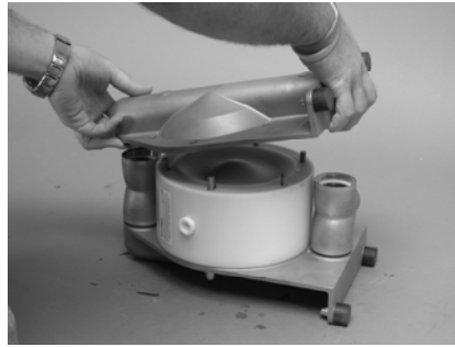
Remove side housing [1] and suction/discharge ports [2].
