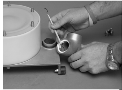
Draw the O-rings port outside [7] off the side housings [1]. Remove the inner O-rings [6] out of the ports [2].
