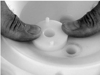
Push out the air-valve housing with the mounting tool turned around.
