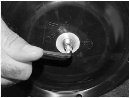
Screw out the set screws, shaft [13a].
