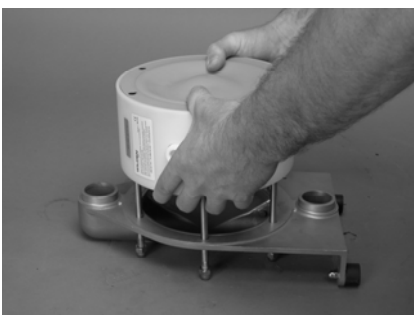
Remove the center block [16] by gently pulling apart.
