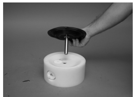
Pull the other diaphragm [14] together with the shaft [13] out of the center block [16].
